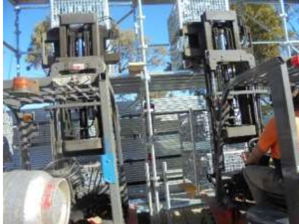
Minimum Strength Load Test Pm with approx. 10.2tonne
